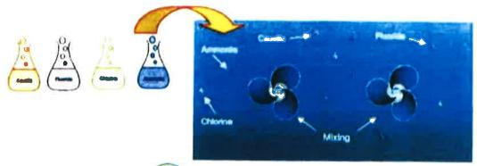
After UV inactivation, the water is treated with a combination of chlorine and ammonia to form a product called chloramine.
