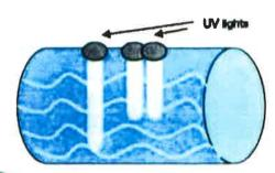
Some organisms in the water, such as Giardia and Cryptosporidium, are resistant to disinfection treatment and therefore must be inactivated. We treat the water with ultraviolet (UV) radiation to inactivate these organisms.
