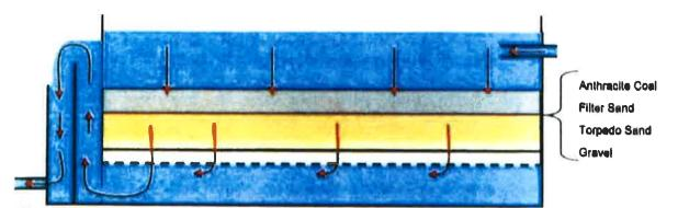
Any particles remaining in the water after coagulation and sedimentation are removed by passing the water through filters made from crushed coal. (anthracite.), sand, and gravel. The filters catch the small particles and do not allow them to pass through the filter.
