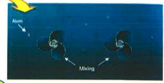
At the water plant the water is treated with a chemical called Aluminum sulfate (alum). Alum is used in a process called coagulation, which helps dirt, bacteria, algae, and other particles bind together and form larger particles called floc. These chemicals are added to the water and mixed using large propeller mixers.
