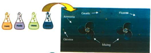
After UV inactivation, the water is treated with a combination of chlorine and ammonia to form a product called chloramine. Chloramines further disinfect the water while hindering the formation of unwanted trihalomethanes (THMs), in addition, Fluoride is added to the water to help protect our teeth from decay, and Caustic is added to help stabilize the pH of the water.
