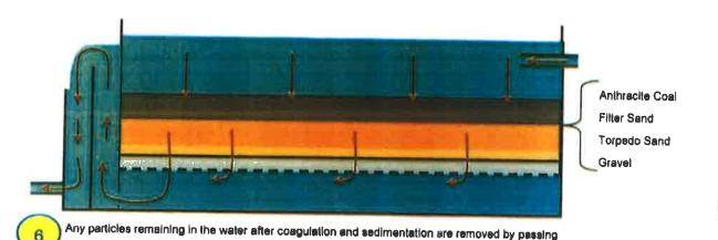
the water through filters made from crushed coal (anthracite), sand, and gravel. The filters
