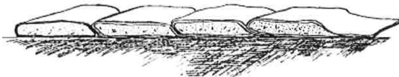
Figure 3 – Overlap sandbags lengthwise and parallel to river flow.
